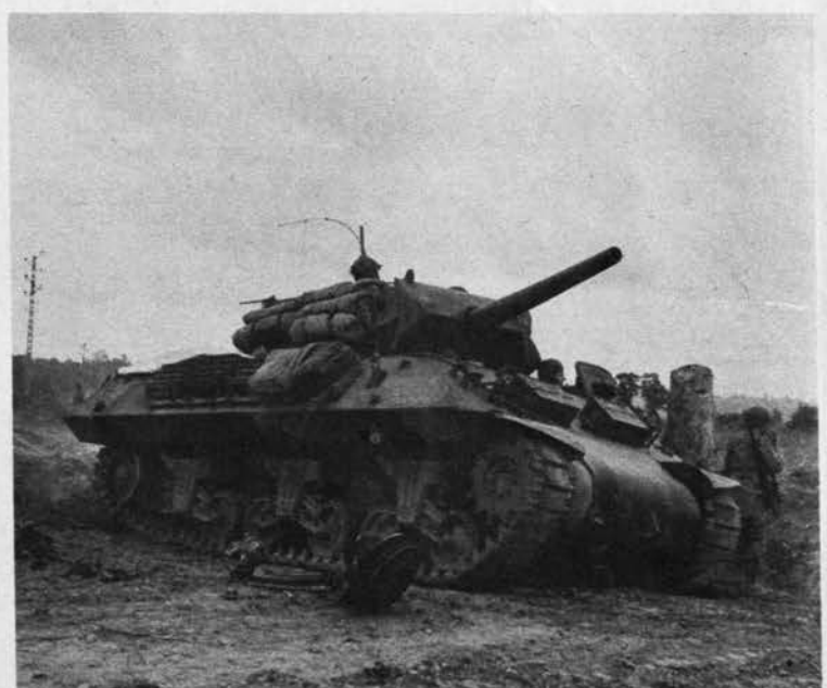
Awaiting orders , the crew of an M-10 get set to roll after the breakthrough beyond St. Lo. Main weapon is a 3-in. gun in a low angular turret mounted on M-4 chassis. Turret has sharply undercut sides.
